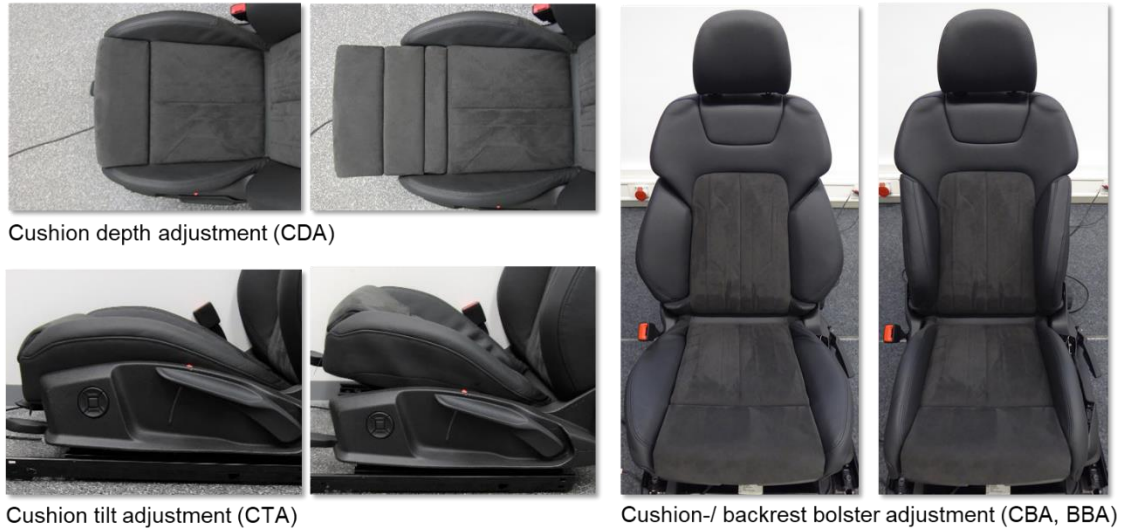
Fig. 1. Experimental seats with modified adjustment tracks.
