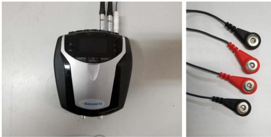
Fig. 4. Mangold-10 wireless Bluetooth multi-channel physiology system made in Germany
