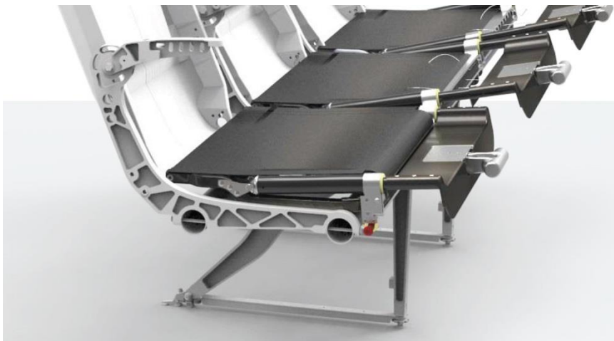
Fig.5. The basic structure of the seat pan developed in this project.
