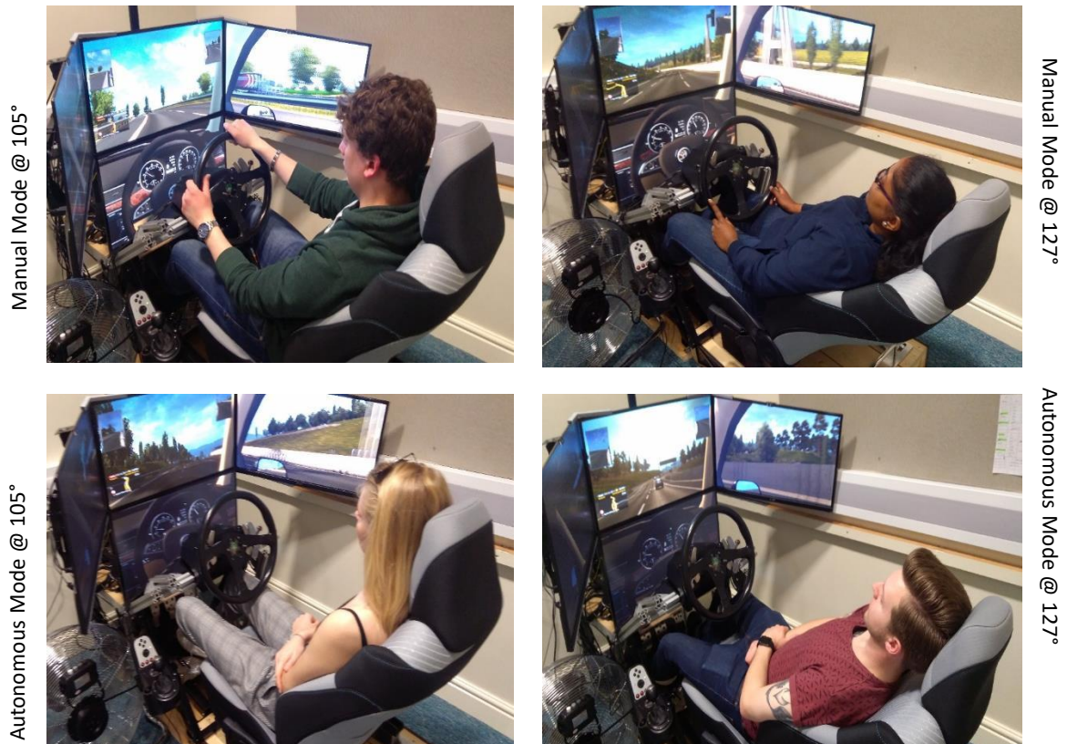
Fig. 2. Lab setup showing manual and autonomous modes in the two driving positions.
