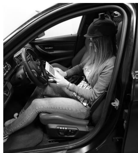
Fig. 2. Occupant in driving simulator with sensors on head, chest, seat cushion and seat rail.
