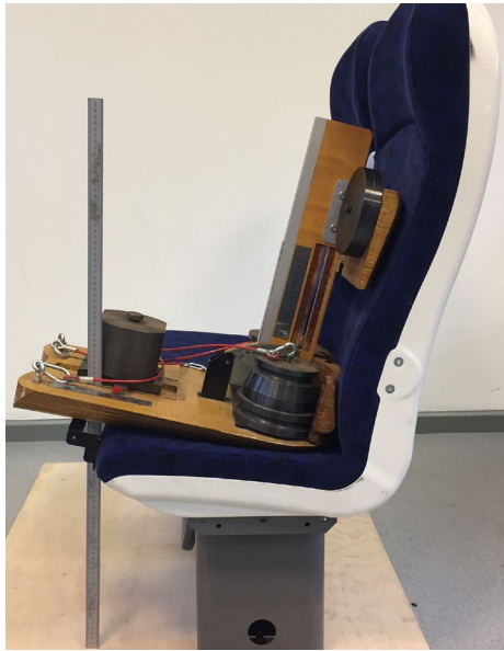
Fig. 1. CMD used to measure seat dimensions (ISO TR 24496:2017).
