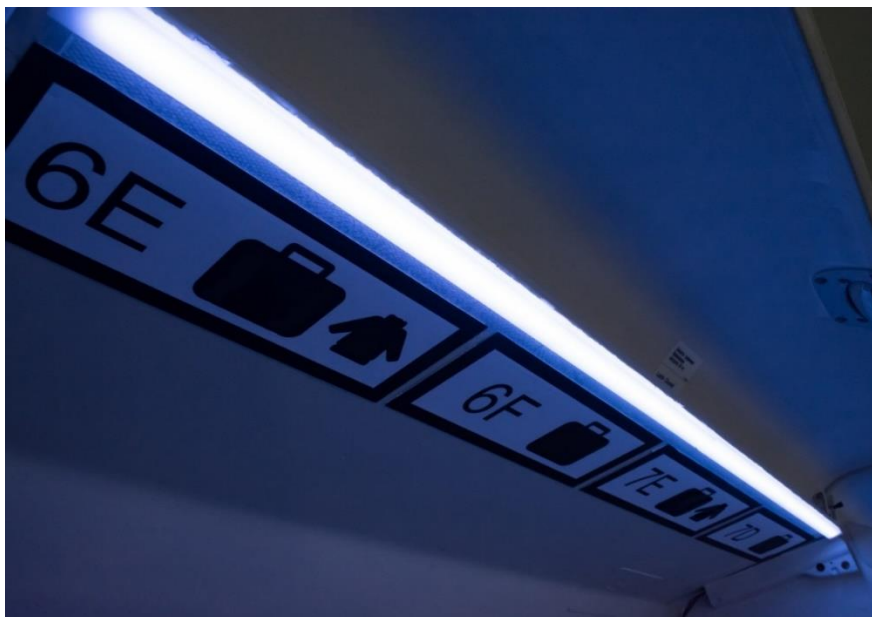
Figure 2. Luggage divisions including a light strip, an outline, seat number, and icon.
