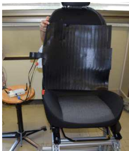
Fig. 3. The Medilogic® Seat Pressure Measurement System placed on the seat
