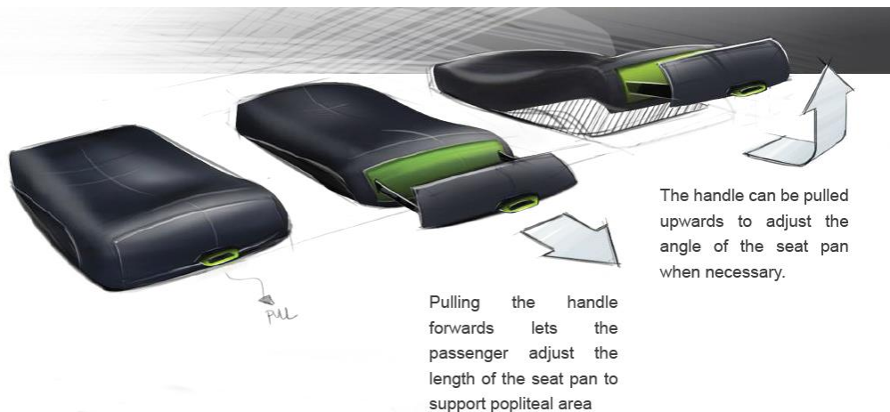
Fig.3. Rough design and working principle of the adjustable seat pan.
