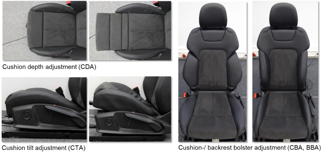
Fig. 1. Experimental seats with modified adjustment tracks.
